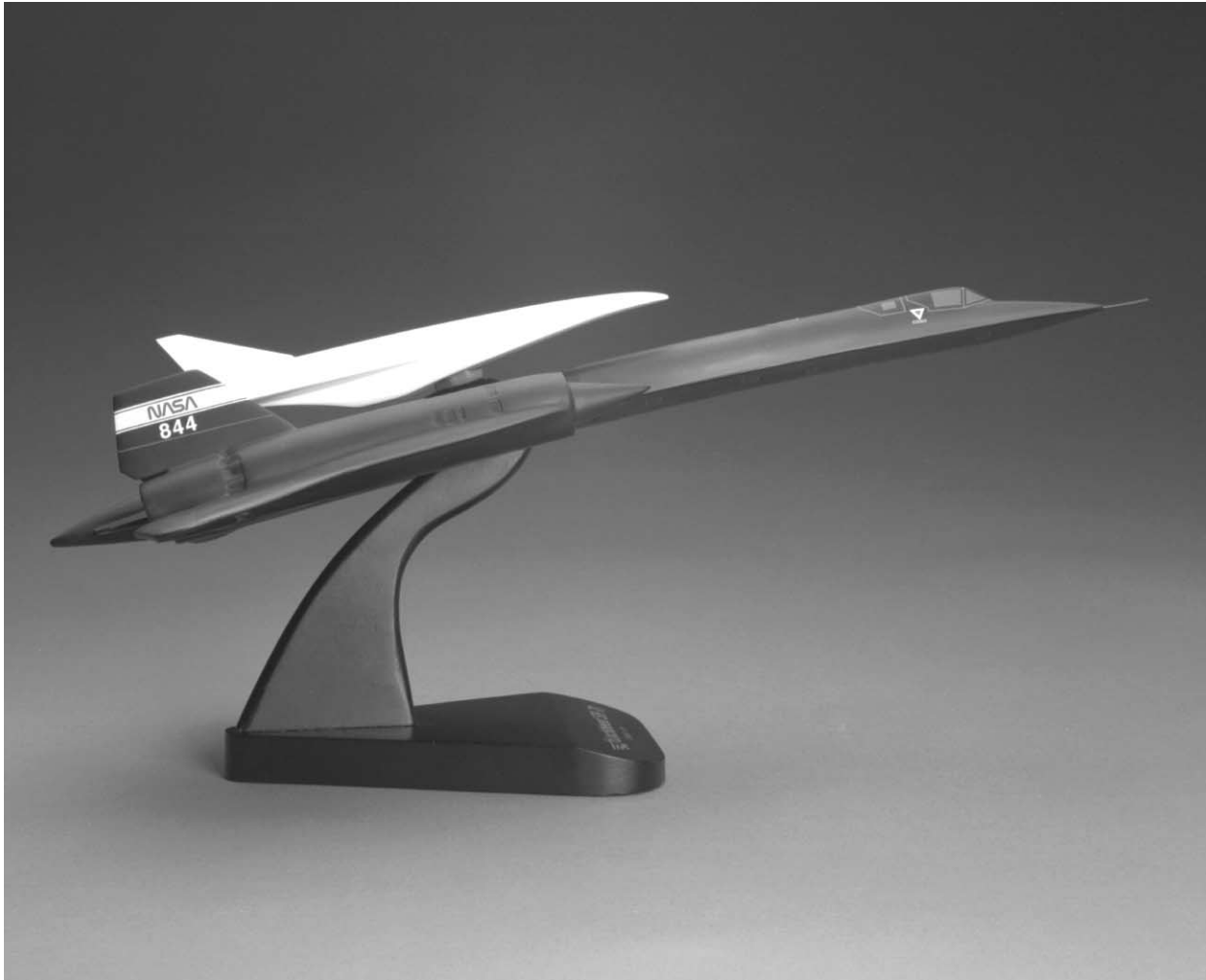
FIGURE 2. MODEL OF THE SR-71 AIRCRAFT AND BACK-MOUNTED GENERIC HYPERSONIC RESEARCH VEHICLE.
